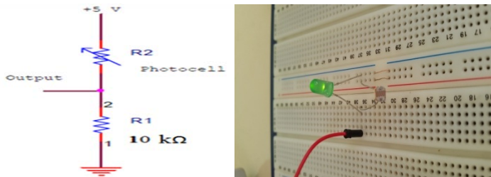
Fig. 5. LDR sensor connected with constant resistor.
